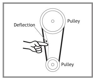
Figure 87. Check for proper belt tension.
